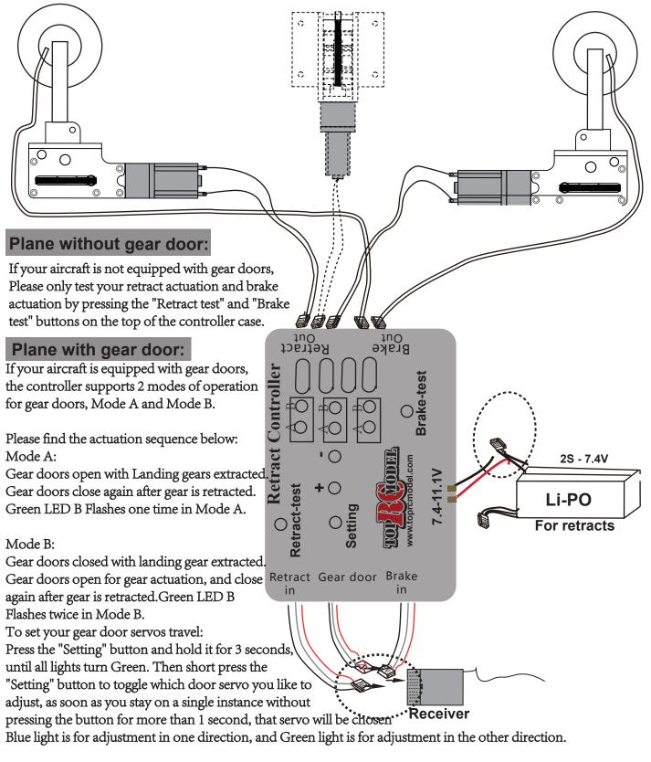
Assemble the landing gear to your aircraft after running several (~5) cycles of gear actuation to verify everything is working correctly and you are fully acquainted with the function of the controller and gears.
