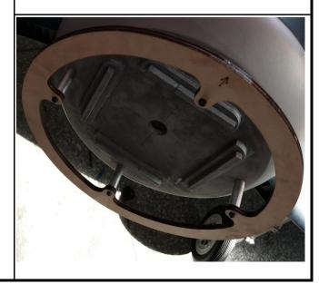
19.Install the engine to the firewall with screws, put the cowling to the engine and glue the cowl to the ply wood frame.
