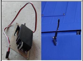
2. Assemble the flap on the outer wing. Prepare the servos for flaps, trim slots to appropriate position in the outer wing and flaps, apply instand type AB glue to the slots in the flaps and horns. Connect the servo to the horn with screws.
