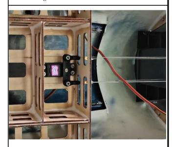
18. Assemble the ply cowl frame to the fuselage.
