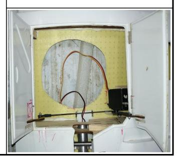
7. Assemble the main retracts and gear cover parts to the retract mount with screws .
