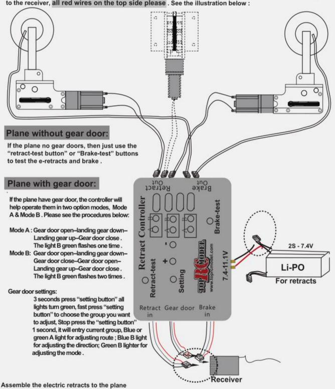
Assemble the electric retracts to the plane after several times smoothly running.
