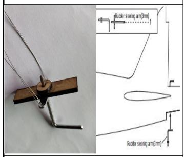
15. Apply AB glue to the slots in the rudder assemble the rudder to the vertical fin of the plane, epoxy the ply wood plate to the fuselage.
