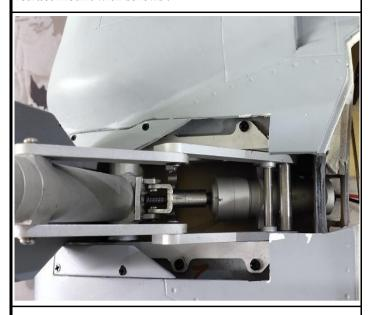
8. The pictures after gear door cover install finished and gear door open .
