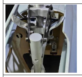
17. Mount the fuel tank. Assemble the servo for rudder in the fuselage and connect them via the steel wire .
