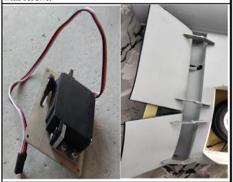
5. Epoxy the pinned hinges, horns to the inner gear door carefully,
