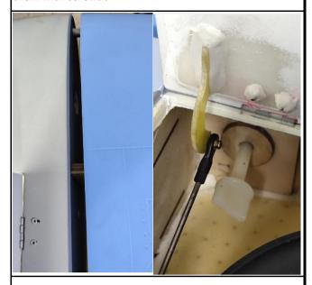
11. Assemble the wing to the fuselage and lock it with screws.
