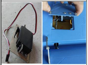
3. Fix the servo to the wing, Keep some space between the trailing edge and the aileron to make sure it can rotate smoothly.
