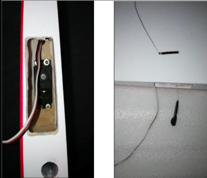
2. Adjust the servo arm to the right position and fixing it to the servo with screw, see picture .
