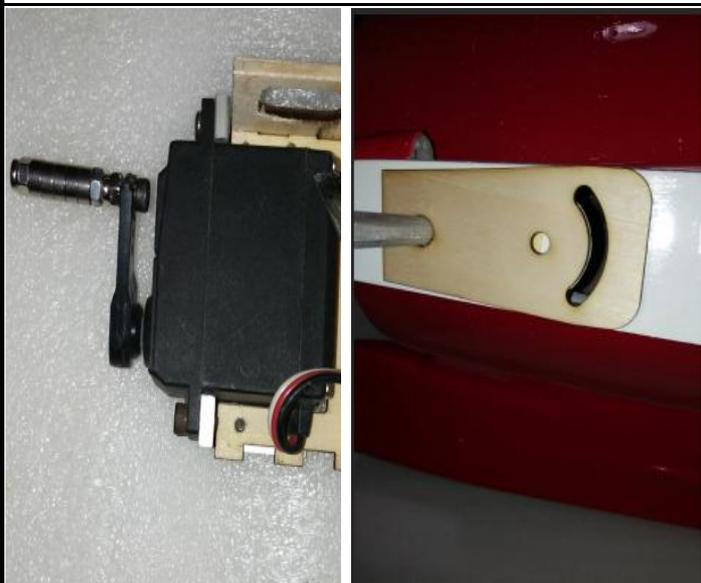
7. Assemble the stab servo to appropriate position in the fuselage with screws and make sure the screw with bearings can move through the slot smoothly .
