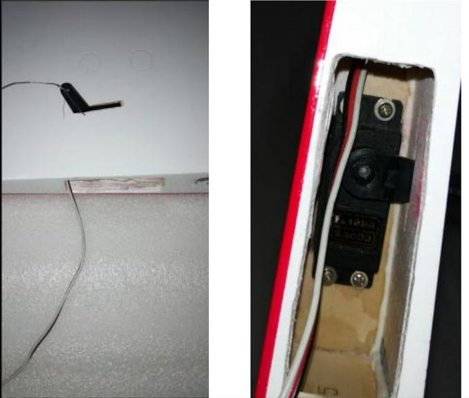
3. Glue the horns to the aileron, Connect the horns to the servo arms with the linkage and lock each side with screws and nut. Make sure the aileron can at least 30mm
