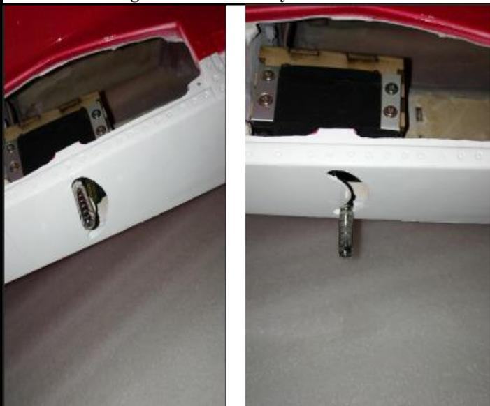
8. Assemble the stab to the fuselage and make sure it can turn freely .
