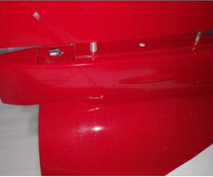
13. Lock the vertical fin by screws from the tail fuselage holes, make sure the rudder can move smoothly .
