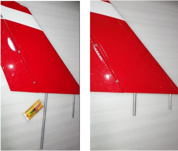
12. Assemble the vertical fin to the tail fuselage .
