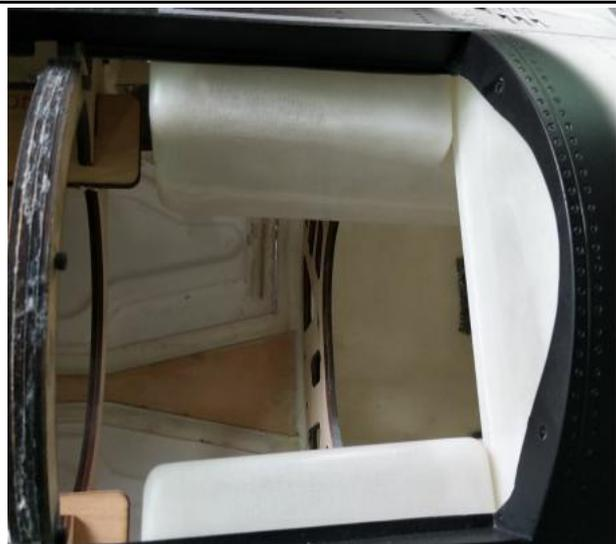
31. When you need to add some accessories under the cockpit, please remove the nose and pull the steel wires.
