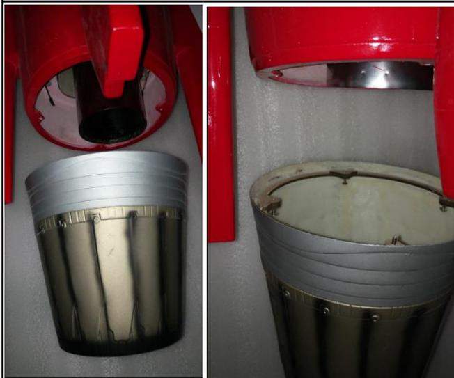
19. Fix the tail pipe through assembly the 3mm ply tail pipe frame, see pictures below .
