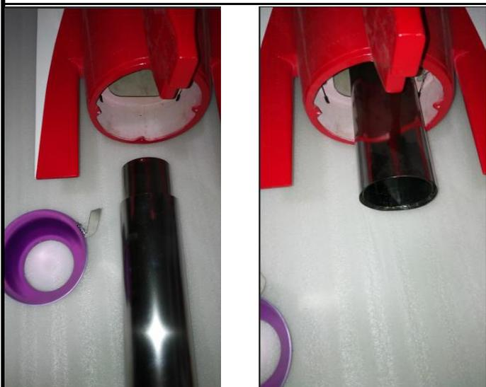
17. Lock pipe socket to the tail pipe with schrews and nut, and fix the side of pipe socket to the fuselage asbelow .
