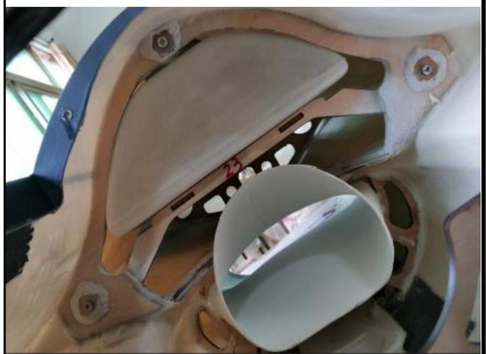
30. Assemble the other two fuel tanks to the main fuselage .
