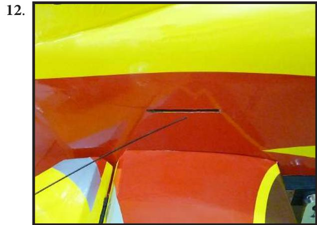
Thread cable through brass swage tube.
