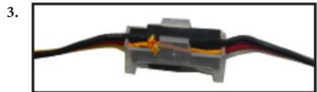
Fasten the pull string from the servo hole to the male plug of the servo extension.
