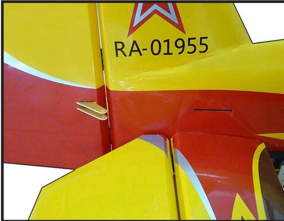
Thread the rudder cable through a brass swage tube, then the threaded coupler, and back through the brass swage tube on both sides. Pull light tension on the cable through the coupler on both sides as shown.
