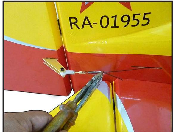
Cut off excess cable as shown.
