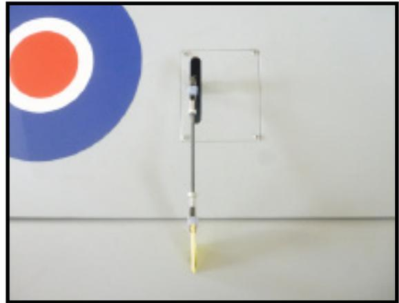
**INSTALLING THE FLAP PUSHROD.**
