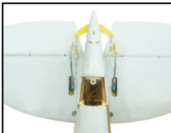
**RUDDER PUSHROD INSTALLATION.**
