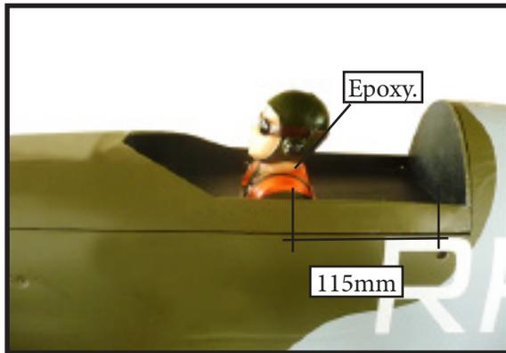
4) Position the canopy onto the fuselage. Trace around the canopy and onto the fuselage using a felt-tipped pen. Carefully cut and remove covering material from the fuselage where the canopy makes contact, exposing the bare wood. Permanently glue the canopy in place with epoxy glue or special "canopy glue".
