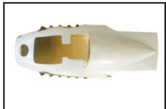
1) Carefully align the cowling on the airplane. The front of the cowl should be positioned so the crankshaft is in the middle of the cowl opening. Hold the cowl firmly in place using pieces of masking tape.
