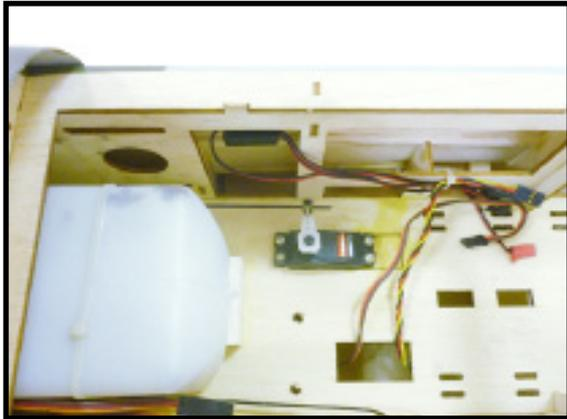
2) Move the throttle stick to the closed position and move the carburetor to closed. Use a 2.5mm hex wrench to tighten the screw that secures the throttle pushrod wire. Make sure to use threadlock on the screw so it does not vibrate loose.
