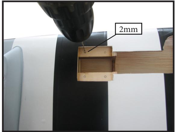
**INSTALLING RETRACTABLE LANDING GEAR.**
