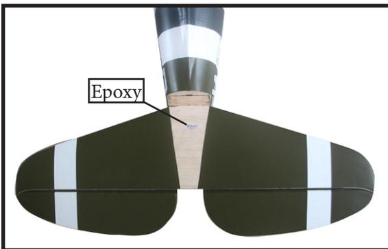
3) Slide the vertical stabilizer back in place. Using a triangle, check to ensure that the vertical stabilizer is aligned 90° to the horizontal stabilizer.
