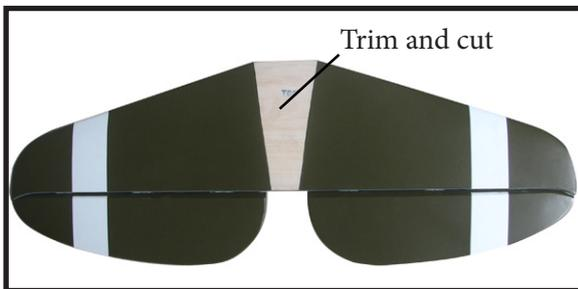
**!** *When cutting through the covering to remove it, cut with only enough pressure to only cut through the covering itself. Cutting into the balsa structure may weaken it.*
