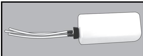
**!** *You should mark which tube is the vent and which is the fuel pickup when you attach fuel tubing to the tubes in the stopper. Once the tank is installed inside the fuselage, it may be difficult to determine which is which.*
