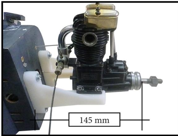
2) Use a pin drill and 4mm drill bit to drill a small indentation in the mount for the engine mounting screw.
