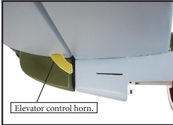
3) Thread one clevis and M2 lock nut on to each elevator control rod. Thread the horns on until they are flush with the ends of the control rods.
