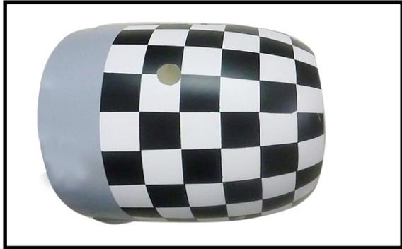
*Because of the size of the cowl, it may be necessary to use a needle valve extension for the high speed needle valve. Make this out of sufficient length 1.5mm wire and install it into the end of the needle valve. Secure the wire in place by tightening the set screw in the side of the needle valve.*
