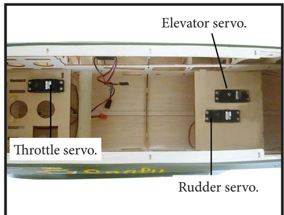
**THROTTLE SERVO ARM INSTALLATION.**
