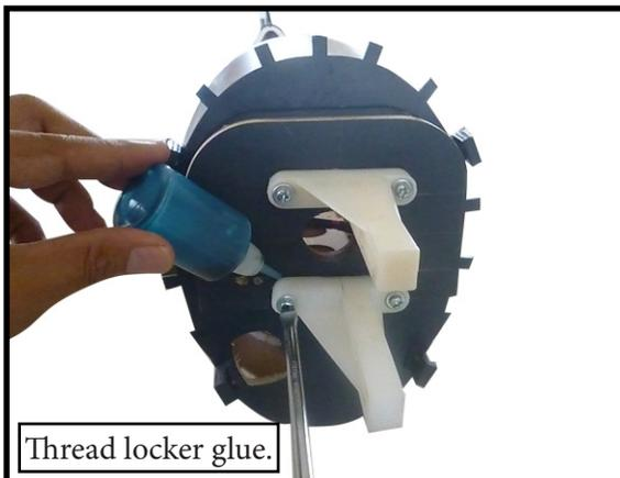
**MOUNTING THE ENGINE - 2 stroke.**
