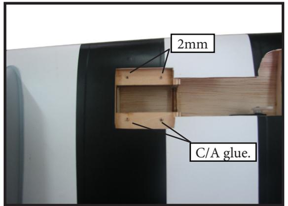
2) Install retractable landing gear at the Wing.
