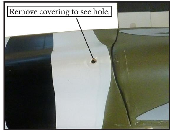
3) Tighten the antenna to the fuselage. The antenna is removeable so you can install it at the flying field to prevent damage in transporting.
