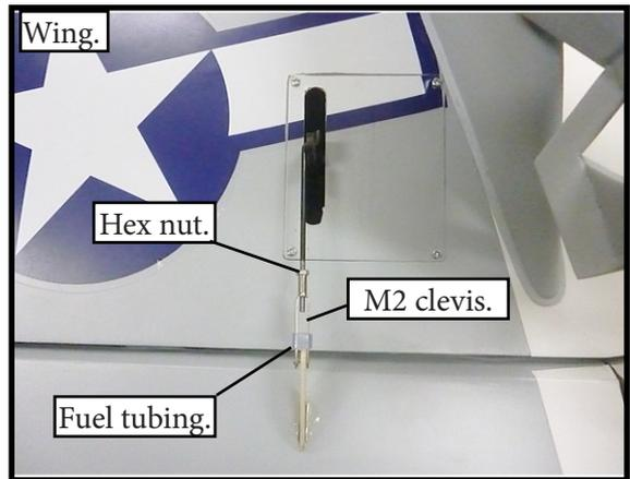
**INSTALLING THE FLAP PUSHROD.**
