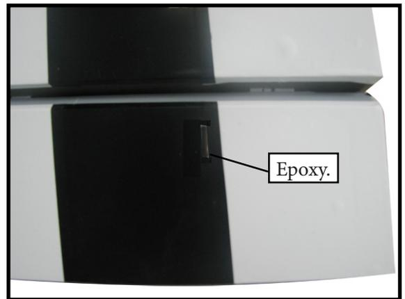
**INSTALL ELEVATOR CONTROL HORN.**
