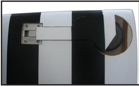
Insert bomb onto the wings.
