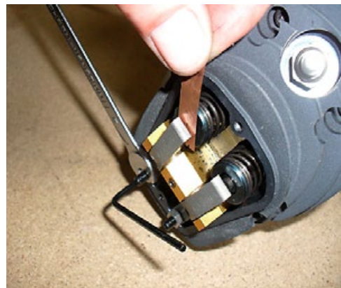
This photo series shows the adjusting of the valve gap with the help of the feeler gauge.
