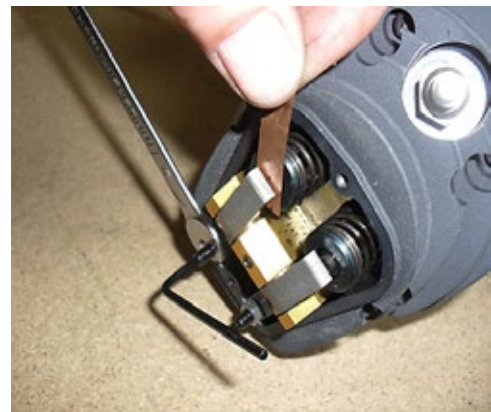
This photo series shows the adjusting of the valve gap with the help of the feeler gauge.
