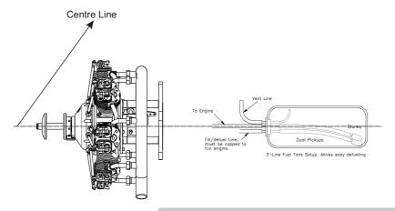
Note: Install the tank on the centre line of the engine
