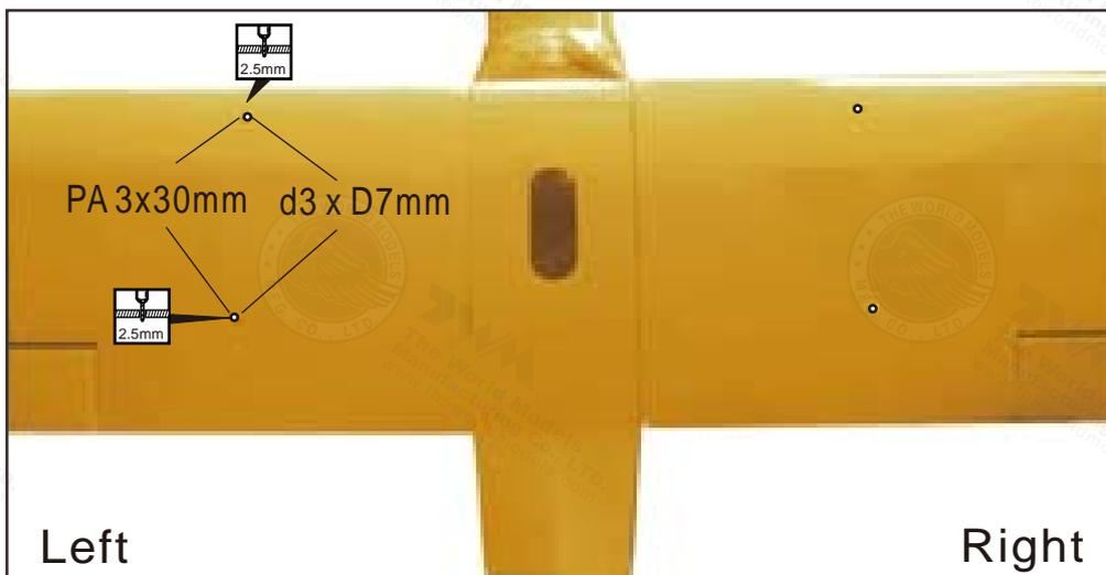
Step 3. Make sure the wings are resting against the fuselage tightly. Locate the pre-drilled 2.5mm hole at top of left wing, and drill along with 2.5mm drill bit until it passes through the wing tube. Apply the PA3x30mm self-tapping screw.
