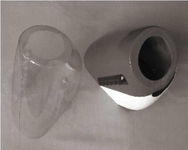
This transparent 3D template is used for position guidance of the actual cutting of the pre-painted cowling.
