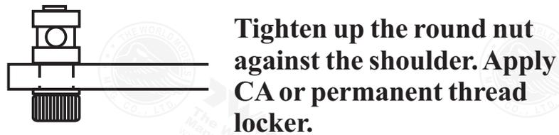
After fastening the round nut, make sure that the linkage connector can rotate freely.
