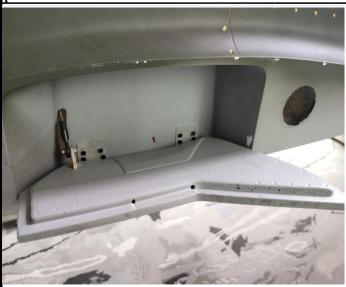
4. Trim slot in appropriate position in wheel house and connect the gear door to the gear door servo, see the pictures.
