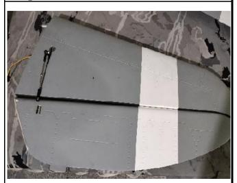
7. Apply AB glue to the slots in the rudder, assemble the rudder to the vertical fin of the plane, connect the rudder and servo by linkage.
