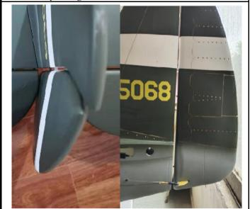
8. Glue one side of the stab tube to one stabilizer, assemble it to the fuselage throught the stab tube, assemble another stabilizer to the fuselage and lock the stabilizer with screw
