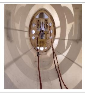
12.Install the fuel tank, servos and controller in the fuselage and make sure they are tightly fixed .
