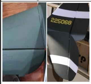
9. Assemble the wings to the fuselage and lock the wings by the clamps which in the fuselage, see picture below.
