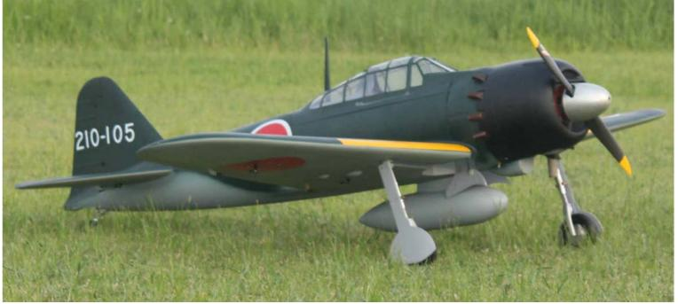
Specification: Wing Span: 2362mm/93in 1916mm/75.4in Length: Flying Weight: 12.3kg Wing area: 93.7dm2 Engine: 60-80cc R/C System: 8+ channel radio system Servo: 10 C.G: 145mm back from the leading edge at wing root
