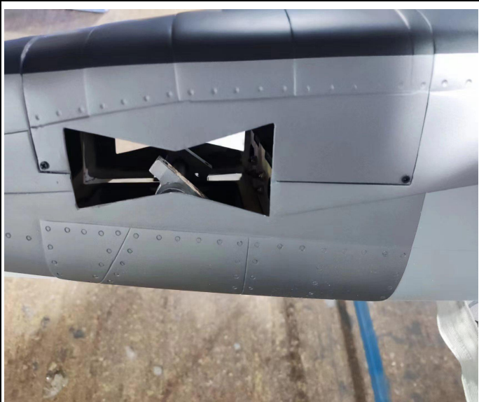
21. Put the pivot & round hinge into the parts
