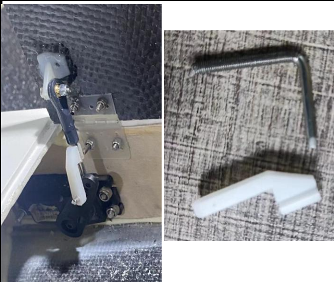
20. Fix the main gear B into the main gear with screw
