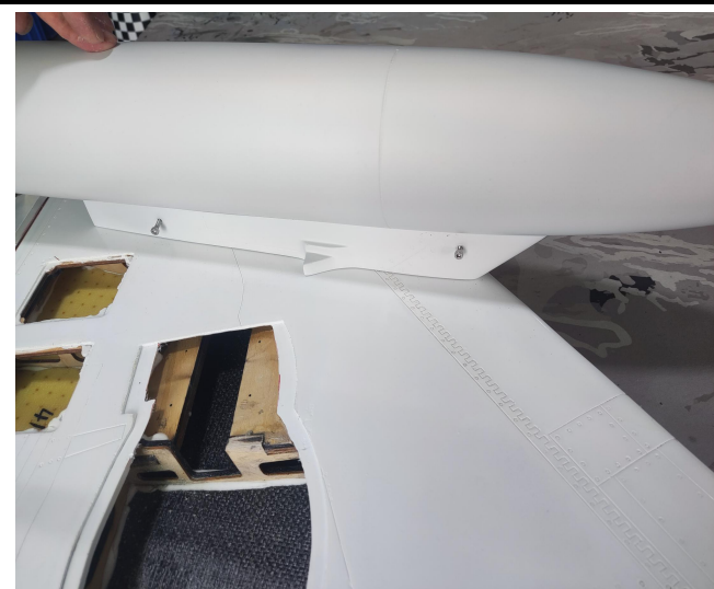
24. Fix the Missile on the rack with screw
