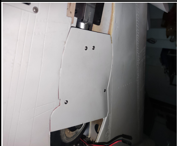
20. Fix the main gear B into the main gear with screw
