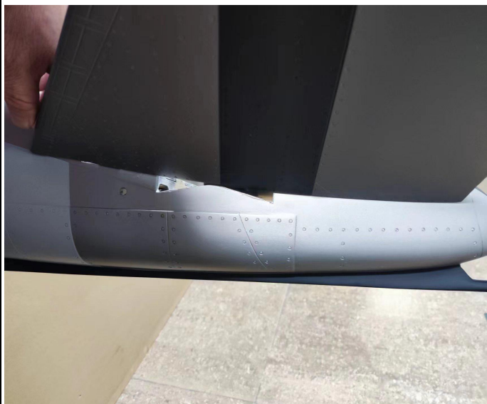
20. Fix the elevator cover with screw.
