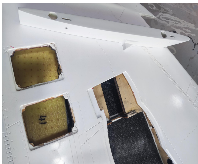
23. Fix the Missile rack on the wing with screw and AB glue.
