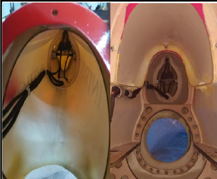
20.Fuselage harnesses done with protective sleeves, and routed .
