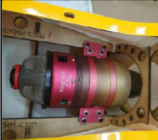
24.Engine seated in place .
