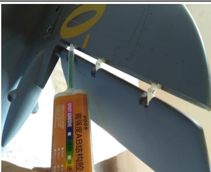
13. Apply instand type AB glue to the holes in the rudder and assemble the rudder to the tail fin.
