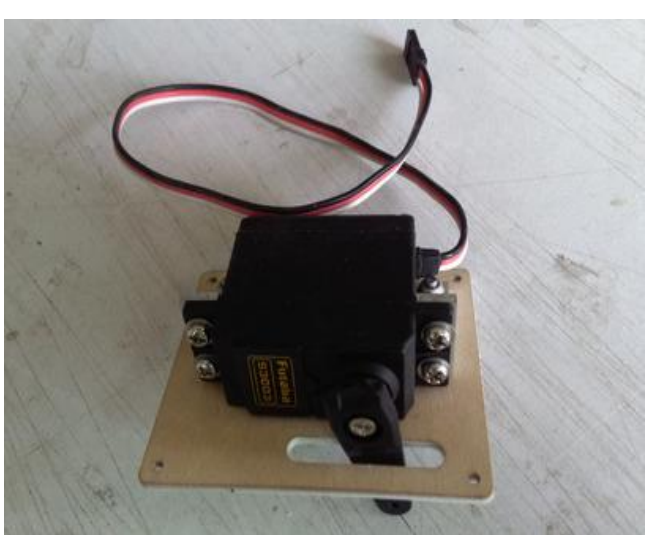
14. Assemble the servos to the stab servo trays and also rudder servo tray.
