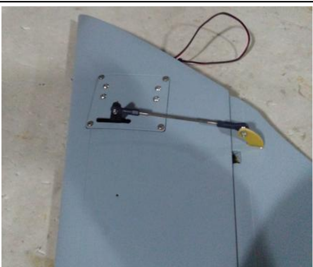
16. Fix the servo trays to the stab with screws, Connect the fiber horns to the servo arms with the linkage and lock each side with screws and locknuts.
