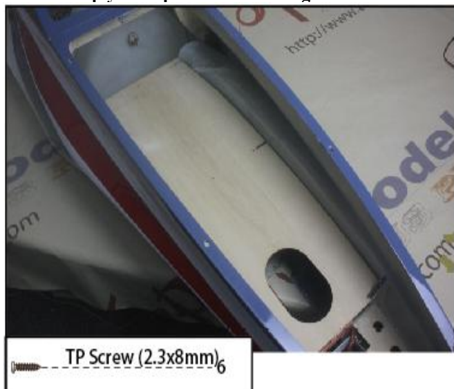
37.Put the plywood plate in the fuselage.
