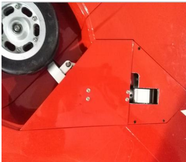
55. Assemble the wheel cover to the main retracts.
