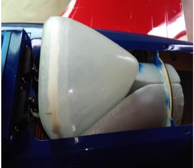
63. Assemble the fuel tank to the fuselage.
