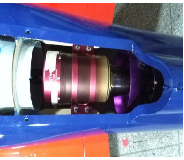
62. Assemble the turbine engine to the fuselage.
