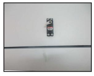
Reinstall the servo into the servo mount and secure the servo inplace using the wood screws provided with you radio system.
