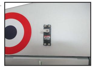
Attach the string to the servo lead and carefully thread it though the wing. Once you have thread the lead throught the wing, remove the string so it can use for
