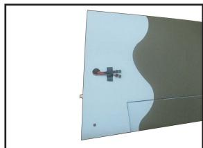
Attach servo lead to the aileron servo.
