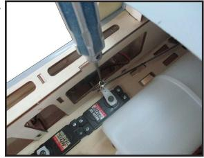
Reinstall the servo horn by sliding the
