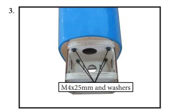
Attach the motor mount to the front of the electric motor box using four 4mm blind nut, four M4x25mm hex head bolts to secure the motor. Please see picture shown.
