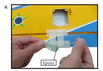
Before the epoxy fully cures, remove the tape from around the control horn. This will allow the epoxy to flow around the control horn, creating a small filet between the control horn and surface for a fiished look and secure bond.
