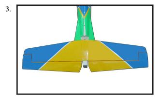
With the stabilizer held firmly in place, use a pen and draw lines onto the stabilizer where it and the fuselage sides meet. Do this on both the right and left sides and top and bottom of the stabilizer.
