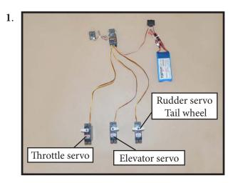
Secure the servos with the screws provided with your radio system.
