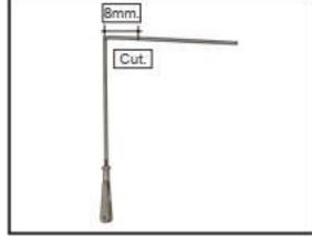
Make a 90-degree bend at the mark and cut off the excess wire leaving 8mm past the bend.
