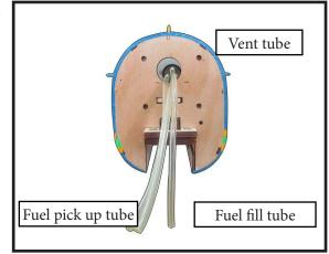
Connect the lines from the tank to the engine and muffler. The vent line will connect to the muffler and the line from the clunk tothe carburetor.
