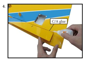
Turn the wing panel over and deflect the flap in the opposite direction from the opposite side. Apply thin C/A glue to each hinge, making sure that the C/A penetrates into both the aileron and wing panel.
