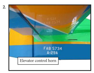
Thead one clevis and M2 lock nut on to each elevator control rod. Thead the horns on until they are flsh with the ends of the control rods. Elevator and rudder pushrods assembly as pictures below.
