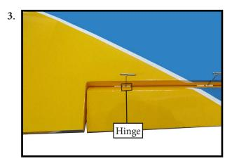
Deflect the aileron and completely saturate each hinge with thin C/A glue. The ailerons front surface should lightly contact the wing during this procedure. Ideally, when the hinges are glued in place, a 1/64" gap or less will be maintained throughout the length of the aileron to the wing panel hinge line.
