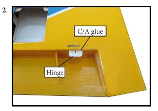
Slide the wing panel on the flap until there is only a slight gap. The hinge is now centered on the wing panel and flap. Remove the T-pins and snug the aileron against the wing panel. A gap of 1/64" or less should be maintained between the wing panel and flap.
