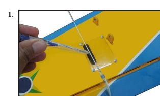
Mark the control wire where it crosses the servo arm hole.
