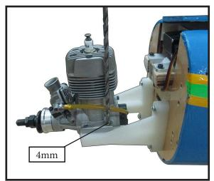
Use a drill to drill the four holes in the engine mount rails.
