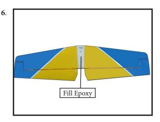
When you are sure that everything is aligned correctly, mix up a generous amount of 30 Minute Epoxy. Apply a thin layer to the top and bottom of the stabilizer mounting area and to the stabilizer mounting platform sides in the fuselage. Slide the stabilizer in place and realign. Double check all of your measurements once more before the epoxy cures. Hold the stabilizer in place with T-pins or masking tape and remove any excess epoxy using a paper towel and rubbing alcohol.
