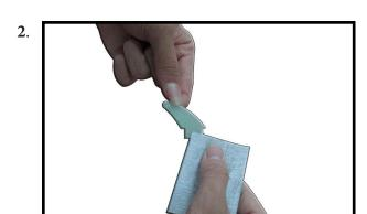
Check the fit of the control horns to the aileron and flap. They should rest flush against the control surface as shown.
