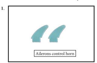
Use sandpaper to scuff the bottom of the aileron and flap control horns. Use a paper towel and isopropyl alcohol to remove any oils or debris from the control horns.
