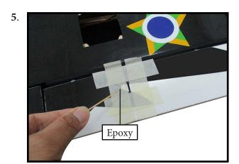
Apply epoxy to the area of the control horns that fist into the slots. Use enough epoxy so the control horns will be fully bonded to the fied surfaces.
