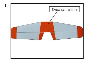
Using a modeling knife, carefully remove the covering at mounting slot of horizontal stabilizer (both side of fuselage).
