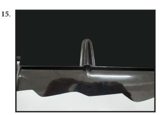
Use canopy glue to attach the cover to the wing. Use low-tack tape to keep the cover in position until the adhesive fully cures.
