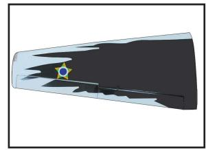
Check the fit of the aileron to the wing. The top of the ailerons will align to the top of the wing. Make sure movement is smooth and bind free.
