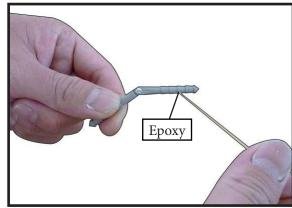
Apply epoxy to each hinge where it will be inserted into the ailerons. Tip: Apply some petroleum jelly to the metal pin hinge area to keep epoxy from interfering with smooth operation of hinge.
