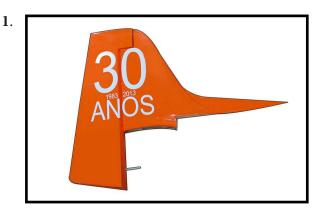
Using a modeling knife, remove the covering from over the precut hinge slot cut into the lower rear portion of the fuselage.
