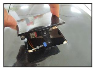
Use a pin vise and 3/32-inch (2mm) drill bit to clear the paint from the flap control horn.
