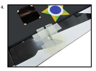
Remove the control horns from the control surfaces. Apply epoxy to the slot in the aileron and flap. Make sure the epoxy gets into the slot for a good bond between the surfaces and control horn.
