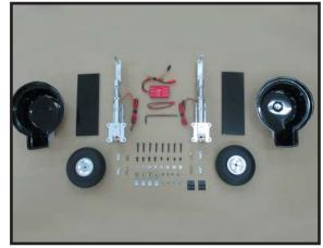
Install retractable landing gear at the Wing.
