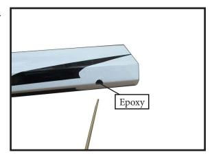
Apply epoxy into each of the holes in the ailerons using a spare piece of pushrod wire or toothpick.
