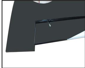
Once adjusted, make sure all clevis retainers are in position. Apply a drop of threadlock near the clevis, then tighten the nut against the clevis to keep the linkage from changing length inside the wing.
