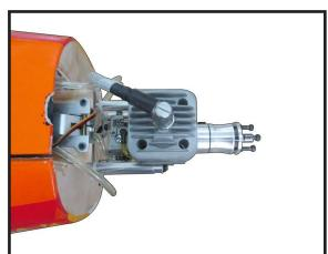
Reinstall the servo horn by sliding the connector over the pushrod wire. Center the throttle stick and trim and install the servo horn perpendiular to the servo center line.
