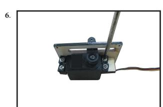
Apply 1-2 drops of thin C/A to each of the mounting tabs. Allow the C/A to cure without using accelerator.
