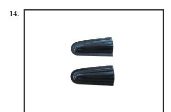
Fit the flap linkage cover into position. Check the operation of the flap to make sure the cover does not interfere with the flap linkage.
