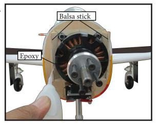
Attach the motor to the front of the electric motor box using four 5mm blind nut, four M4x20mm hex head bolts to secure the motor. Please see picture shown.
