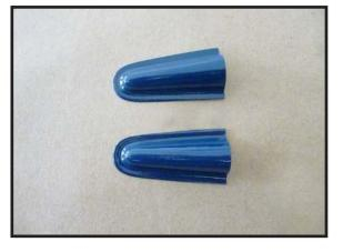
Fit the flap linkage cover into position. Check the operation of the flap to make sure the cover does not interfere with the flap linkage.
