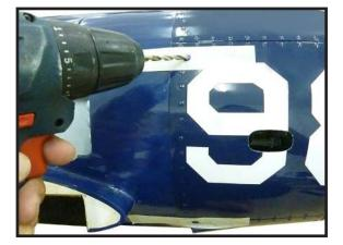
Install the muffler and muffler extension onto the engine and make the cutout in the cowl for muffler clearance. Connect the fuel and pressure lines to the carburetor, muffler and fuel filer valve. Secure the cowl to fuselage using the M4x25mm socket head screws.Putting a small length of silicon fuel tube under the head of the screw helps with vibration.
