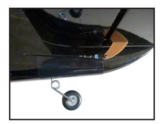
Insert wood piece to the back fuselage as shown.
