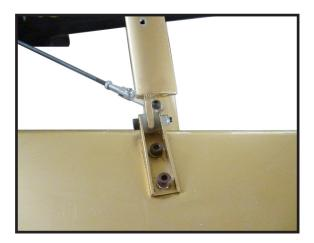
Attach the mounting bracket to the rear diagonal brace using an M3 x 15 socket head cap screw, two nylon washers and an M3 lock nut.
