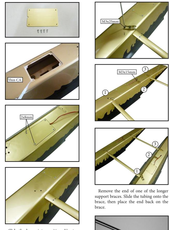
Slide the brace into position. Use two M3 x 25 socket head screws and a 2.5mm hex wrench to attach the mounting bracket and brace in the flat in both position 1 &3. And use M3x15 for position 2.
