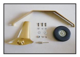
1) Using the hardware provided, mount the main landing gear to the fuselage.
