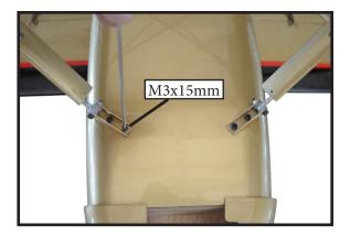
Attach the rear brackets to the fuselage using four M3 x 15 socket head cap screws and a 2.5mm hex wrench.
