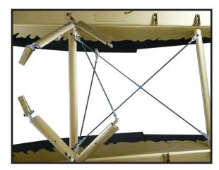
Attach the front cross brace wire to the front diagonal brace using an M3 x 15 socket head cap screw, two nylon washers and an M3 lock nut.
