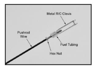
Use a felt tip pen to mark the wire where it crosses the hole. Use a pair of pliers to put a shrp 90-degree bend in the wire at the mark.
