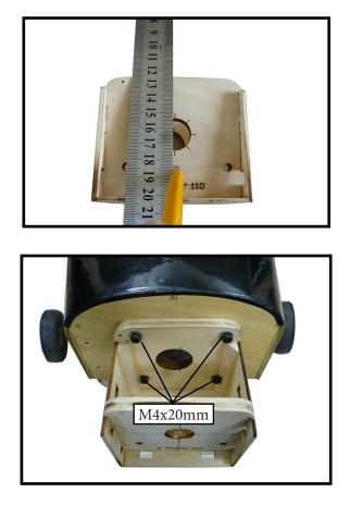
4) Attach the motor to the front of the electric motor box using four 4mm blind nut, four M4x20mm hex head bolts to secure the motor. Please see picture shown.
