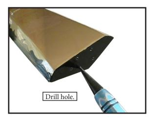
Place 2 to 3 drops of thin CA in each hole to harden the surrounding wood. Allow the CA to fully cure before proceeding.
