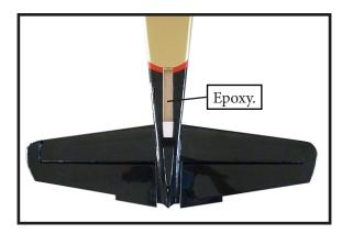
2) Slide the vertical stabilizer back inplace. Using a triangle, check to ensure that the vertical stabilizer is aligned 90° to the horizontal stabilizer.
