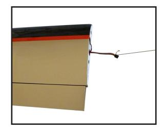
2) Tape the servo lead to the wing to prevent it from falling back into the wing
