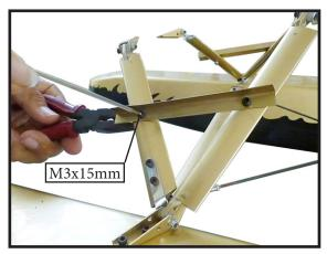
NOTE : Leave the screw slightly loose until the floats are attached to the fuselage.
