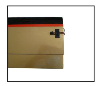
3) Set the aileron servo in place and use a Phillips screw driver to install it with four wood screws.
