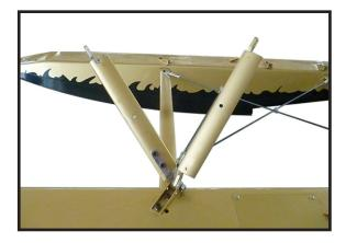
Attach the mounting bracket to the front diagonal brace using an M3 x 15 socket head cap screw, two nylon washers and an M3 lock nut.
