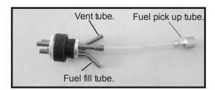
3) Carefully bend the second tube up at a 45° angle. This tube is the vent tube.
