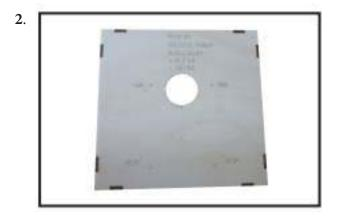
Use a 1/4 bit to drill the engine mounting holes. Remove mounting template from fie wall. Firewall shown with mounting holes drilled ready for engine mounting. Using mounting bolts and washers mount engine to fiewall.
