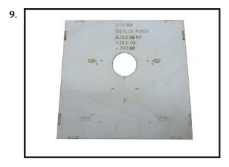
Use a 1/4 bit to drill the engine mounting holes. Remove mounting template from fie wall. Firewall shown with mounting holes drilled ready for engine mounting.
