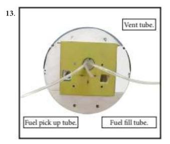
Connect the lines from the tank to the en gine and muffler. e vent line will connect to the muffler and the line from the clunk to the carburetor.
