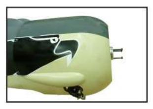
Install the muffler and muffler extension onto the engine and make the cutout in the cowl for muffler clearance. Connect the fuel and pressure lines to the carburetor, muffler and fuel filler valve. Secure the cowl to fuse lage using the M3x10mm socket head screws.
