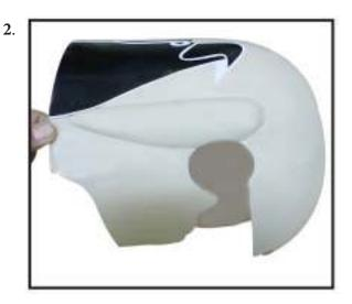
Tape the cowl to the fuselage using low-tack tape.
