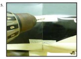
With the muffler, needle valve, and spark/ glow plug removed from the engine, slide the cowl in place over the engine. Temporarily install the propeller and spinner in order to find the exact location of the cowl. Whensatisfied with the cowl placement, secure the cowl to the fuselage using masking tape.
