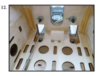
Drill a hole for the throttle pushrod.
