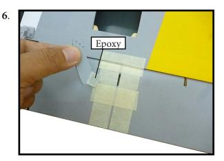
Before the epoxy fully cures, remove the tape from around the control horn. This will allow the epoxy to flow around the control horn, creating a small filet between the control horn and surface for a filshed look and secure bond.
