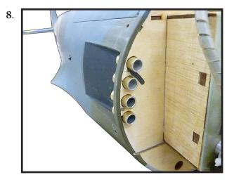
Locate the laser cut engine mounting template. Align mounting template to front of firewall.
