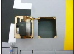
Set the aileron hatch in place and use a Phillips screw driver to install it with four wood screws.
