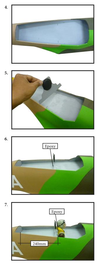
Position the canopy to the fuselage. Trace around the tree canopy and onto the fuselage with a marker. Carefully cut and remove the covering material from the fuselage where the canopy touches, exposing the bare wood. Then screw it in place.
