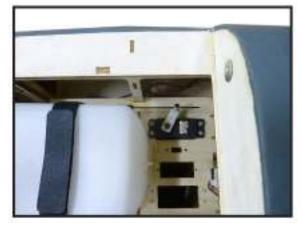
Move the throttle stick to the closed position and move the carburetor to closed.
