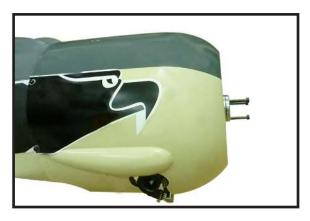
4) Install the muffler and muffler extension onto the engine and make the cutout in the cowl for muffler clearance. Connect the fuel and pressure lines to the carburetor, muffler and fuel filler valve. Secure the cowl to fuselage using the M3x10mm socket head screws.
