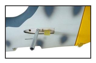
Use Epoxy Glue to glue the Horizontal Stabilizer to the fuselage.
