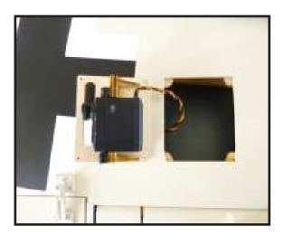
9) Set the aileron hatch in place and use a Phillips screw driver to install it with four wood screws.
