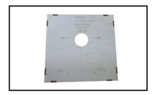
Use a 1/4 bit to drill the engine mounting holes. Remove mounting template from fiewall. Firewall shown with mounting holes drilled ready for engine mounting.
