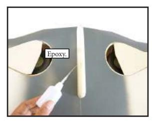
Insert the wing gun onto the wing.
