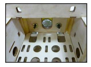
8) Drill a hole for the throttle pushrod.
