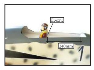
4) Position the canopy onto the fuselage. Trace around the canopy and onto the fuselage using a felt-tipped pen. Carefully cut and remove covering material from the fuselage where the canopy makes contact, exposing the bare wood. Then permanently glue the canopy in place with epoxy glue or special "canopy glue".
