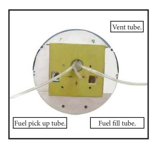
9) Connect the lines from the tank to the engine and muffler. The vent line will connect to the muffler and the line from the clunk to the carburetor.
