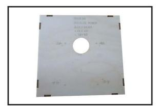
Use a 1/4 bit to drill the engine mounting holes. Remove mounting template from fiewall. Firewall shown with mounting holes drilled ready for engine mounting.
