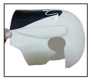
1) Tape the cowl to the fuselage using low-tack tape.
