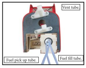
$\Box$  9) Connect the lines from the tank to the engine and muffler. The vent line will connect to the muffler and the line from the clunk to the carburetor.
