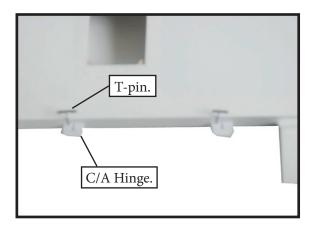
□ 3) Slide the aileron on the wing panel until there is only a slight gap. The hinge is now centered on the wing panel and aileron. Remove the T-pins and snug the aileron against the wing panel. A gap of 1/64" or less should be maintained between the wing panel and aileron.
