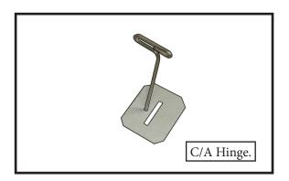
□ 2) Remove each hinge from the wing panel and a leron and place a T-pin in the center of each hinge. Slide each hinge into the aileron until the T-pin is snug against the aileron. This will help ensure an equal amount of hinge is on either side of the hinge line when the aileron is mounted to the wing panel.
