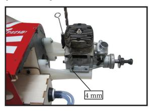
$\square$  3) Use a drill to drill the four holes in the engine mount rails.
