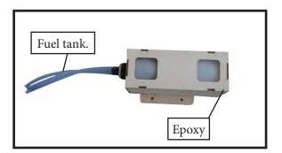
□ 8) Use plywood template to hold in place the fuel tank with C/A glue to secure the fuel tank inside the fuselage.
