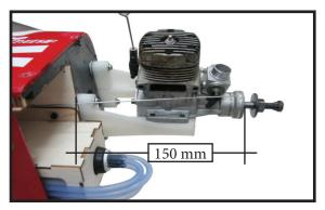
$\square$  2) Use a pin drill and 4mm drill bit to drill a small indentation in the mount for the engine mounting screw.
