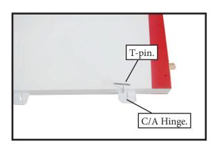
□ 3) Slide the flap on the wing panel until there is only a slight gap. The hinge is now centered on the wing panel and flap. Remove the T-pins and snug the flap against the wing panel. A gap of 1/64" or less should be maintained between the wing panel and flap.
