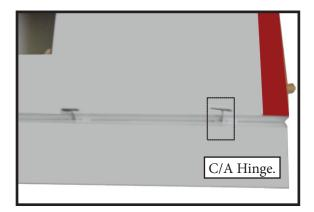
□ 4)Deflect the flap and completely saturate each hinge with thin C/A glue. The ailerons front surface should lightly contact the wing during this procedure. Ideally, when the The hinge are glued in place, a 1/64" gap or less will be maintained throughout the length of the flap to the wing panel hinge line.
