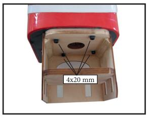
$\square$  3) Attach the motor to the front of the electric motor box using four 4mm blind nut, four M3x15mm hex head bolts to secure the motor. Please see picture shown.
