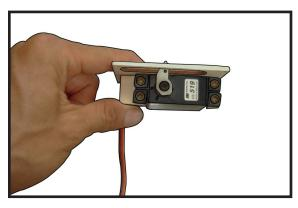
$\Box$  3) Use drill bit in a pin vise to drill the mouting holes in the blocks.
