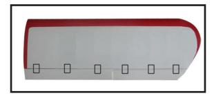
**Note:** Work the aileron up and down several times to "work in" the hinges and check for proper movement.
