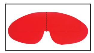
□ 2) Using a modeling knife, carefully remove the covering at mounting slot of horizontal stabilizer (both side of fuselage).
