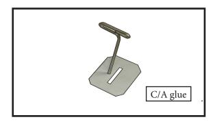
□ 2) Remove each hinge from the wing panel and flap and place a T-pin in the center of each hinge. Slide each hinge into the aileron until the T-pin is snug against the aileron. This will help ensure an equal amount of hinge is on either side of the hinge line when the flap is mounted to the wing panel.
