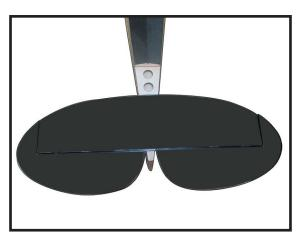
With the stabilizer held firmly in place, use a pen and draw lines onto the stabilizer where it and the fuselage sides meet. Do this on both the right and left sides and top and bottom of the stabilizer.
