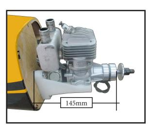
Use a pin drill and 4mm drill bit to drill a small indentation in the mount for the engine mounting screw.
