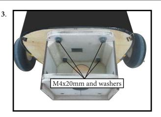
Attach the motor to the front of the electric motor box using four 4mm blind nut, four M4x20mm hex head bolts to secure the motor. Please see picture shown.
