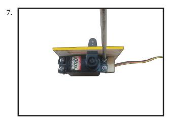
Apply 1-2 drops of thin C/A to each of the mounting tabs. Allow the C/A to cure without using accelerator.
