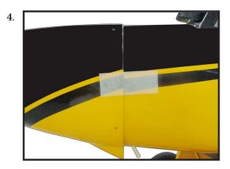
Use a drill and drill bit to drill the holes for the cowl mounting screws. Make sure the cowl position is correct before drilling each hole.
