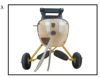
Position the engine with the drive washer (145mm) forward of the fiewall as shown.
