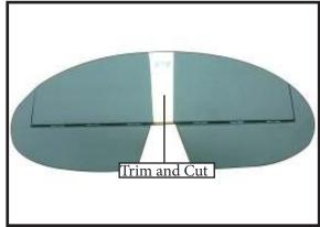
When cutting through the covering to remove it, cut with only enough pressure to only cut through the covering itself. Cutting into the balsa structure may weaken it.
