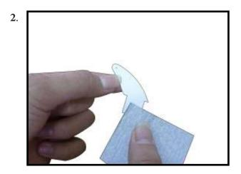
Check the fit of the control horns to the aileron and flap. They should rest flush against the control surface as shown.
