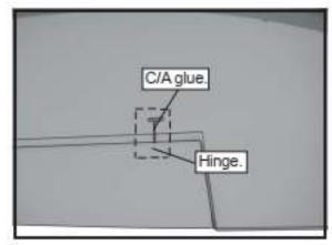
Deflect the aileron and completely saturate each hinge with thin C/A glue. The ailerons front surface should lightly contact the wing during this procedure. Ideally, when the hinges are glued in place, a 1/64" gap or less will be maintained throughout the lengh of the aileron to the wing panel hinge line.
