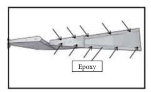
Slide the vertical stabilizer into the slot in the top of the fuselage. The rear edge of the stabilizer should be flush with the rear edge of the fuselage and the lower rudder hinge should engage the precut hinge slot in the lower fuselage. The bottom edge of the stabilizer should also be firmly pushed against the top of the horizontal stabilizer.
