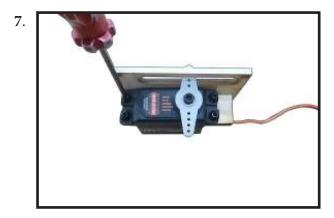
Apply 1-2 drops of thin C/A to each of the mounting tabs. Allow the C/A to cure without using accelerator.
