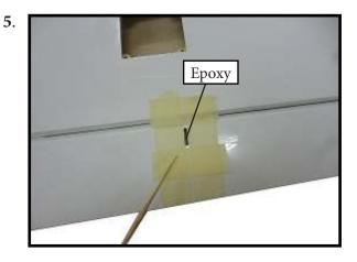
Apply epoxy to the area of the control horns that fist into the slots. Use enough epoxy so the control horns will be fully bonded to the fied surfaces.
