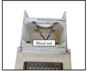
Attach the motor mount to the front of the electric motor box using four 4mm blind nut, four M6x25mm hex head bolts to secure the motor. Please see picture shown.
