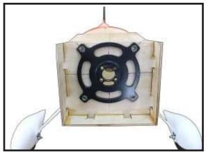
Then, use 8mm drill bit to enlarge the holes on the electric motor box.
