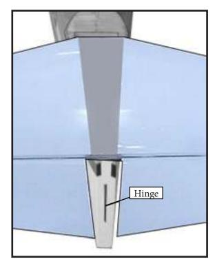
While holding the vertical stabilizer firmly in place, use a pen and draw a line on each side of the vertical stabilizer where it meets the top of the fuselage.
