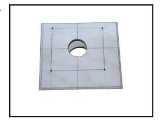
Attach the electric motor box to the firewall centered with the cross lines drawn on the electric motor box and firewall. Using M6x25mm to secure the motor box to the firewall. Please see pictures below.
