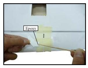
Before the epoxy fully cures, remove the tape from around the control horn. This will allow the epoxy to flow around the control horn, creating a small filet between the control horn and surface for a fiished look and secure bond.
