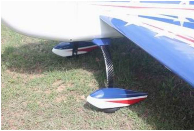
Carbon fiber tail wheel assembly with CNC machined metal parts, including the aluminium tail wheel hub.
