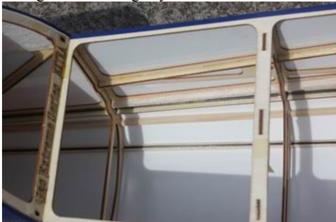
Strengthened fuselage by carbon fiber rods
