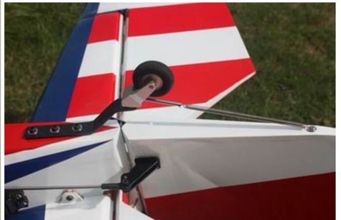
Carbon fiber tail wheel assembly with CNC machined metal parts, including the aluminium tail wheel hub.
