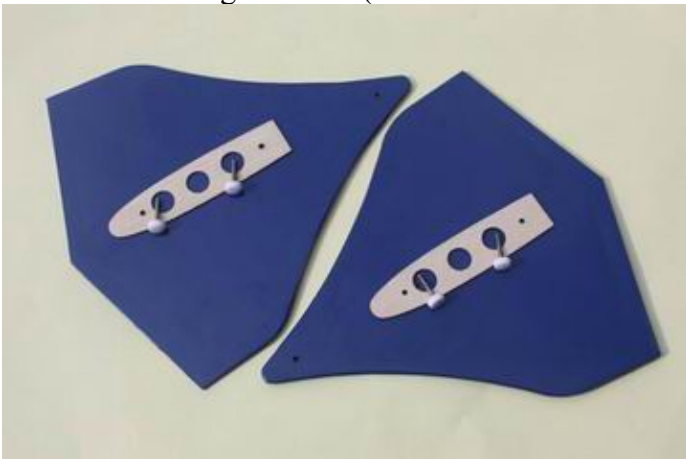
Side force generators (mounted with four M3X18 hand bolts and 2 balsa sheets)
