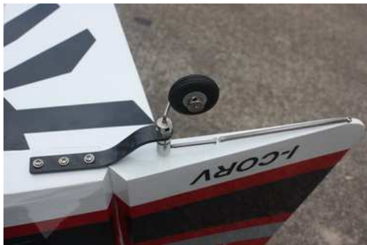
New Carbon fiber tail wheel assembly
