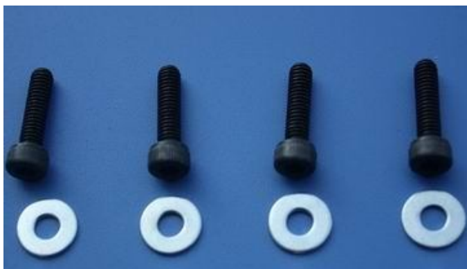
Screws for landing gear: 4(4x20mm) Hexagon bolts & washers
