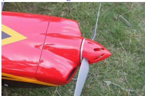
KUZA Alloy Backplate Hollowed-out Electric Spinner included for 90E version (Excellent cooling effect for brushless motor)
