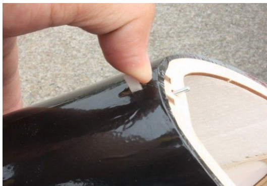
Canopy quick release mechanism
