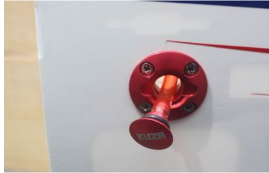
* KUZA CNC Alloy Fuel Vent Line Plug 3 color to choose: black, blue, red No. KAG0232B or KAG0232U or KAG0232R
