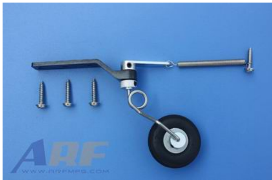
New Carbon fiber tail wheel assembly
