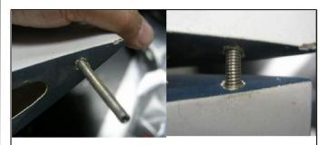
notice:double check and made sure both flap panel can be moving together by spring but will not jam before you glue the flap hinges
